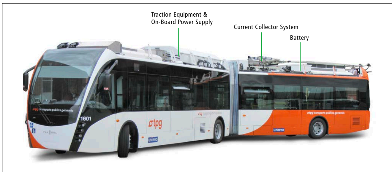
The battery is located under the poles of the current collector system
